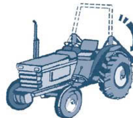
Foldable or manually adjustable (two-post ROPS that fold or telescope for low clearance)
