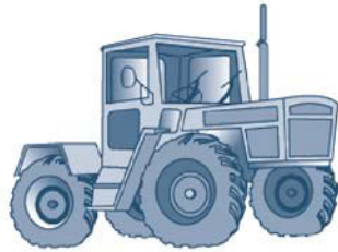
Enclosed cab (cab frame serves as ROPS)
