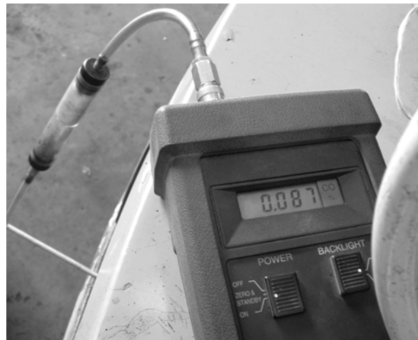
In-house forklift emissions testing.
