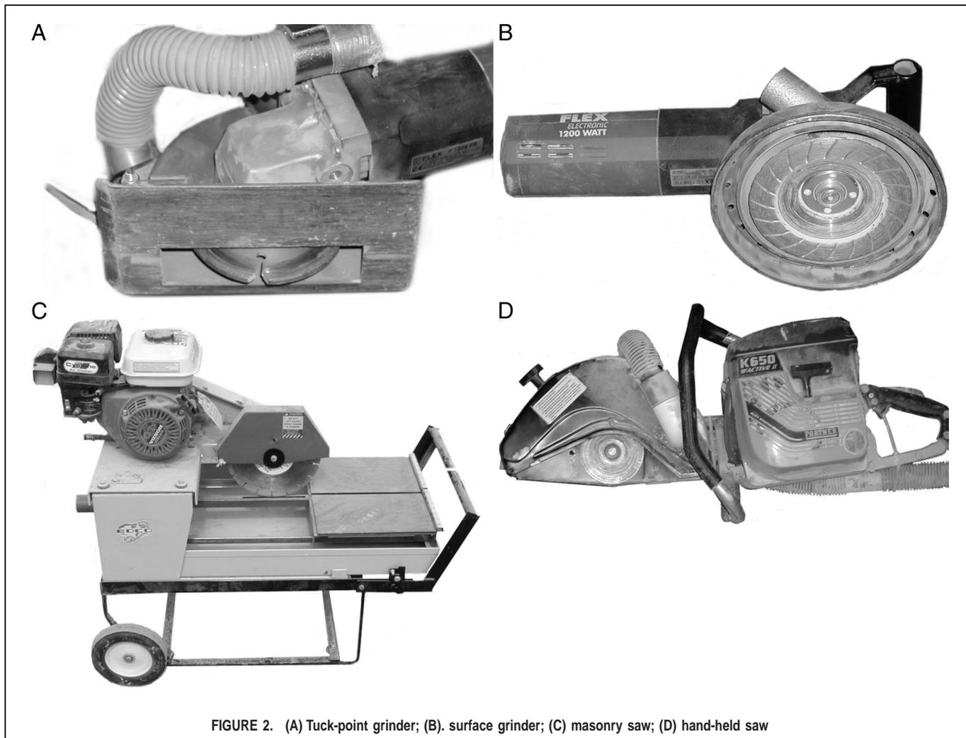
FIGURE 2. (A) Tuck-point grinder; (B) surface grinder; (C) masonry saw; (D) hand-held saw
