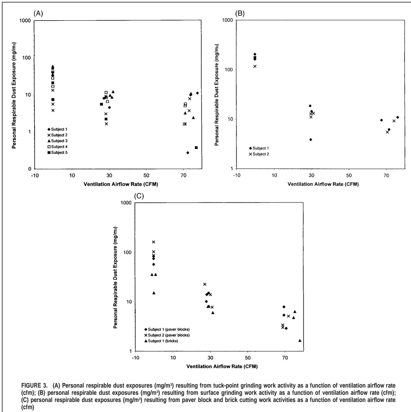
FIGURE 3. (A) Personal respirable dust exposures (mg/m<sup>3</sup>) resulting from tuck-point grinding work activity as a function of ventilation airflow rate (cfm); (B) personal respirable dust exposures (mg/m<sup>3</sup>) resulting from surface grinding work activity as a function of ventilation airflow rate (cfm); (C) personal respirable dust exposures (mg/m<sup>3</sup>) resulting from paver block and brick cutting work activities as a function of ventilation airflow rate (cfm)
