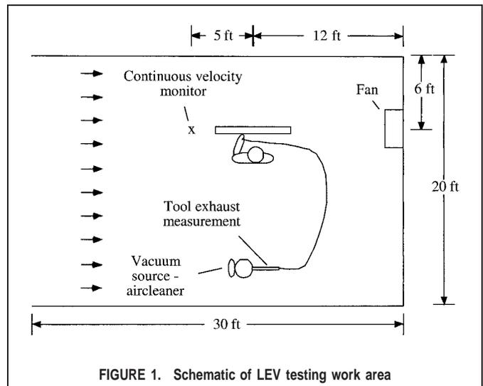
tools (surface grinder, angle grinder, hand-held saw, and masonry saw) equipped with commercially available LEV systems for reducing respirable dust and crystalline silica exposure under controlled field conditions.
