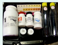
► Figure 2. The Quick Arsenic field test kit. There are Reaction Bottle, three of Quick Reagent, and test strips in the kit.
