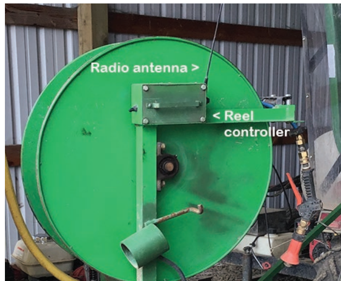
Radio controller installed on hose reel.
