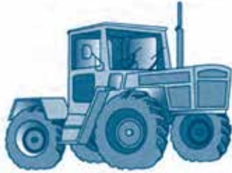
Enclosed cab (cab frame serves as ROPS)
