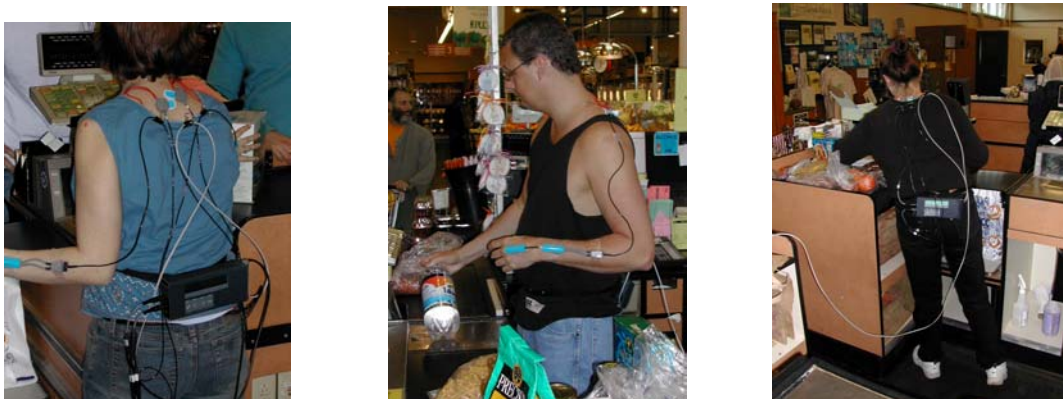
Figure 3. Study equipment: Photo 1 - data logger, trapezius EMG; Photo 2 - left electrogoniometer; Photo 3 - data logger connected by cable to laptop computer
