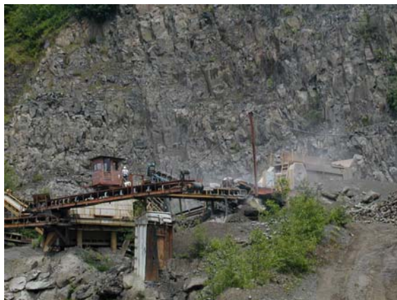
Figure 4: Crusher operator's booth at basalt excavation mine
