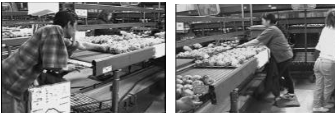
Figure 13 Box Filling and Apple Arranging – Semi-automatic Tray Packing
