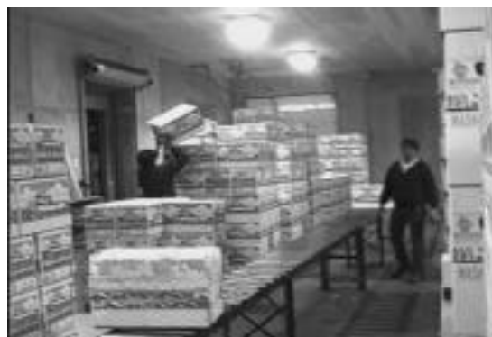
Figure 4 Segregator Stacking Box on Top Layer of Pallet
