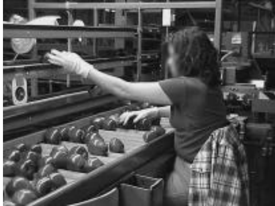
Figure 2 Sorter with Extended Reach to Place Apple on Conveyor
