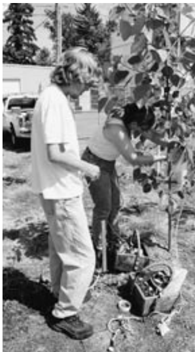
University of Washington students Allan Gross and Marietta Sharp measure contaminants transpired by poplar trees on the Kitsap Peninsula. The Keyport Project uses plants to stop solvents from moving from a Navy landfill to protected wetlands.
